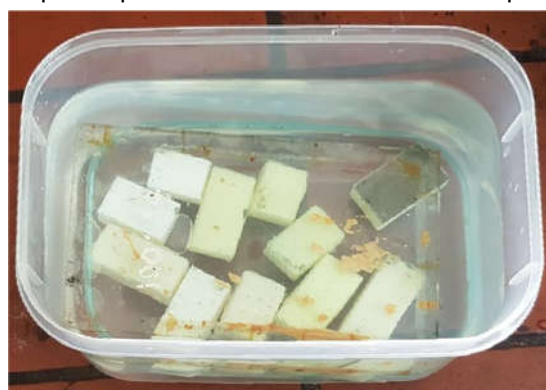
Figure 3. Testing for determination of seawater absorption
