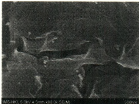
Figure 2. SEM picture of GO
