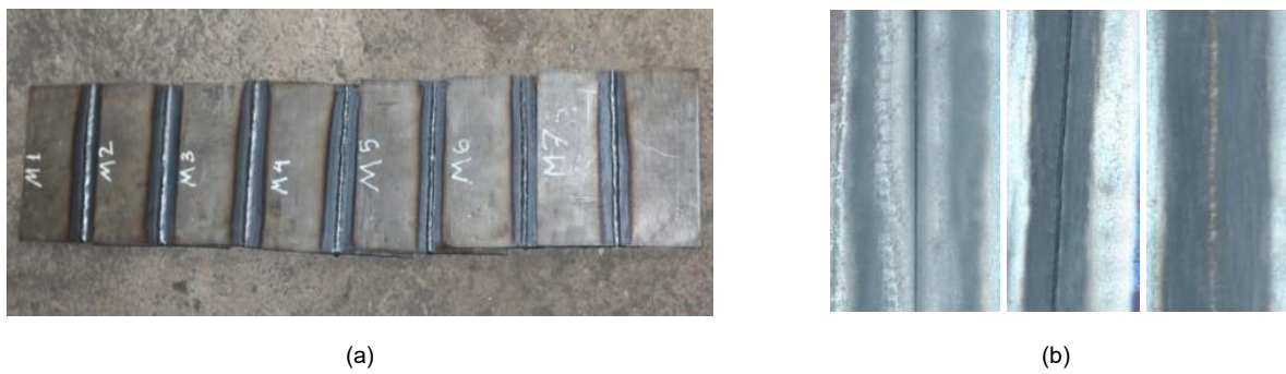
Note: a - The front side of the welded joints; b - The back side of the welded joints.
