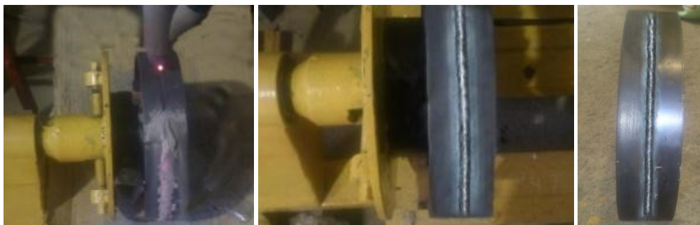
Figure 19. Welding process with sample based on fixture manufactured
