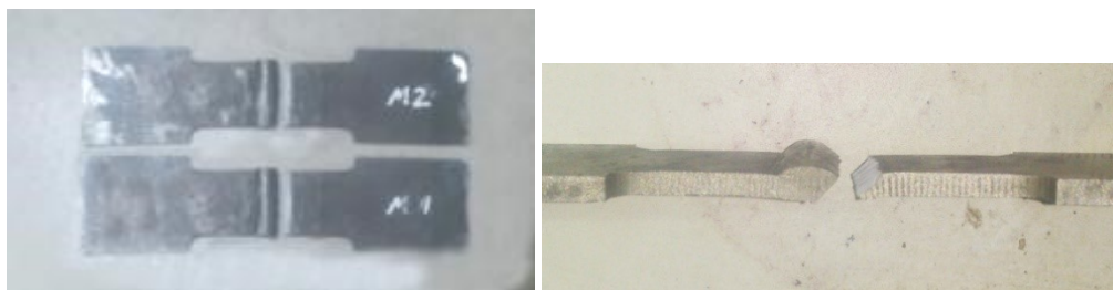
Figure 15. Pieces after the tensile test
