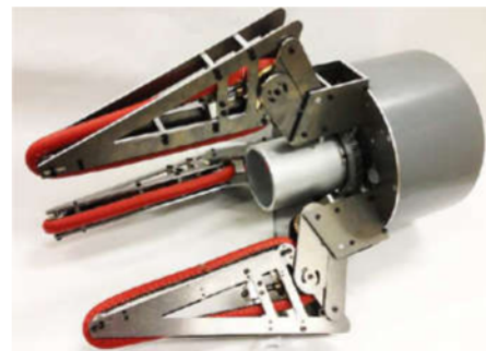
Figure 1. Robotic gripper with three under-actuated finger modules [1]
