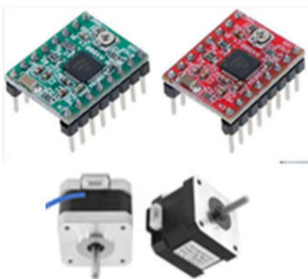
Figure 13. A4988 stepper driver and engines
