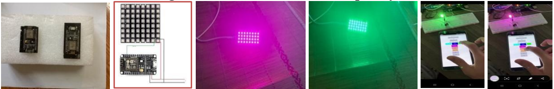
Figure 6. Students make LED lights that connect to Wifi and control via smartphone
