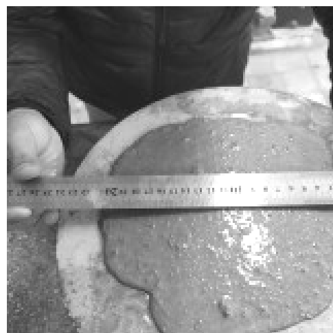
Figure 2. Slump-flow test on SCM mixture at fresh state
