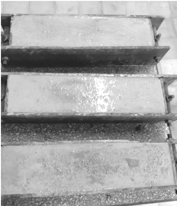
Figure 3. Casting of SCM mixture into the prism mold
