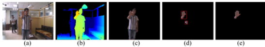
Figure 3. Hand detection and segmentation procedures. (a) RGB image; (b) Depth image; (c) Extracted human body; (d) Hand candidates
